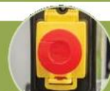
EMERGENCY POWER OFF SWITCH (ALL MODELS)
